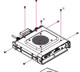
5. Carefully lift the top cover of the main body.
